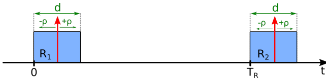
Figure 1: Duty-cycled communication. A device schedules its reception windows R_1, R_2, \dots with an interval T_R . Another device aims to transmit packets within the centers of the reception windows, which is aggravated by a clock skew of \rho \leq \rho_m between sender and receiver.
