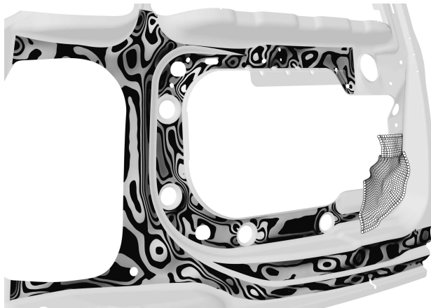
(b) Resulting surface quality (overall reflection pattern and control points for selected patches).
