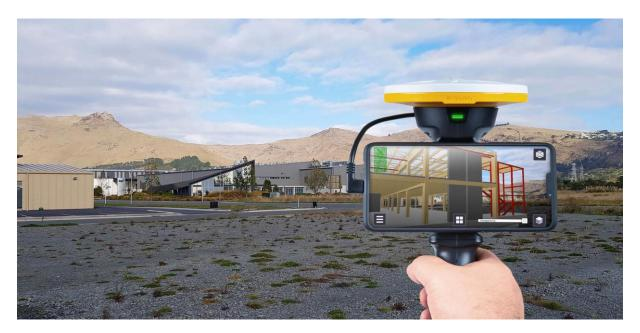
Figure 3.13: Example of Trimble SiteVision (Extracted from:https://sitevision.trimble.com/)
