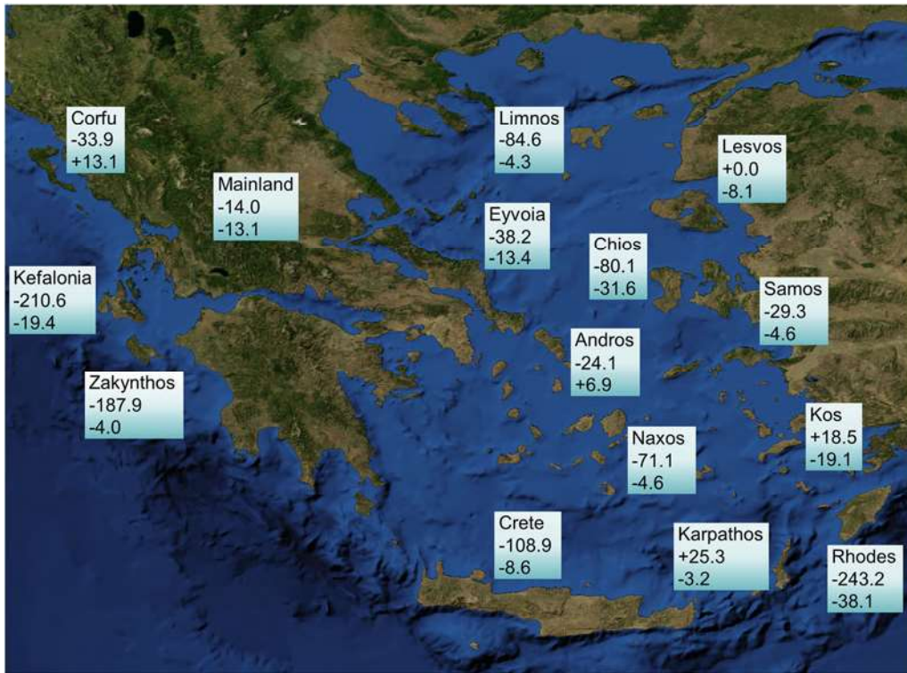
Fig. 3 Mean offset of GOCO05s and extended GOCO05s geoid models to point-wise GPS-levelling observations. The two values give the mean offset of the LVD when calculating the model with EGM and RTM above degree 200 (case 2, bottom value) and without them (case 1, upper value)
