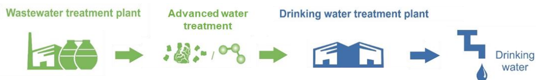
Figure 2-3: A schematic illustration of direct potable reuse (modified from © Berlin Water Company / Technical University of Munich, 2017).
