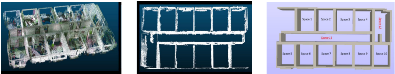
Figure 3.4: Generating geometric digital twins of a building (Ioannis Brilakis' presentation at the workshop)
