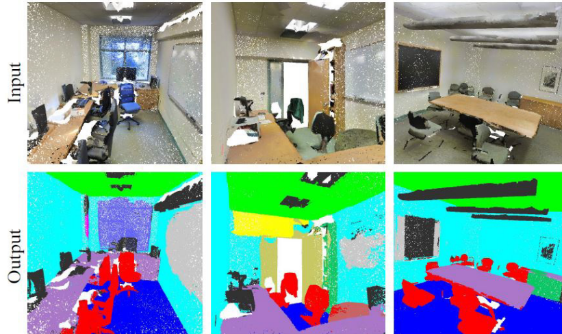
Figure 3.2: One example of point cloud semantic segmentation by deep learning (Qi et al. 2017)
