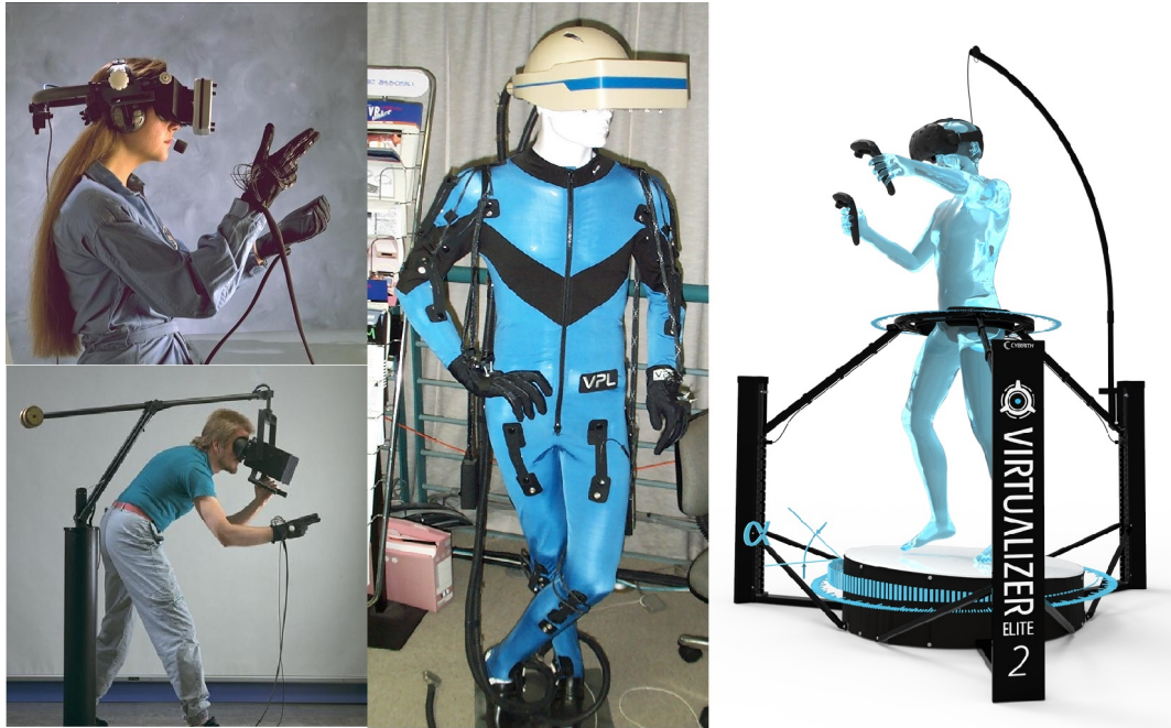
Fig. 2.15. VR design concepts for navigation and interaction. (left) Two strategies of interaction in VR using gloves with sensors. Image on top-left shows mobile HMD and image in bottom-left shows VR headset connected to robotic arm. Author: NASA National Aeronautics and Space Administration, Source: Wikimedia Commons. (center) VR suit A VPL Research DataSuit: a full-body outfit with sensors for measuring the movement of arms, legs, and trunk. Developed circa 1989. Displayed at the Nissho Iwai showroom in Tokyo Author: Dave Pape, Source: Wikimedia Commons, License: Public domain. (right) Virtualizer Elite: VR concept for simulating naturalistic movement for navigation and handheld controllers for interaction in the virtual world.
