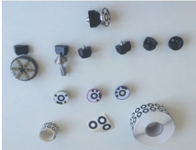
Fig. 3.6. The image shows two types of markers used in the industrial scenario. Markers with encoded patterns are uniquely identifiable which makes image processing and feature matching easy. The image also shows specialized mounts used to place encoded markers on the industrial parts. These mounts are magnetic and their design is customized to be used in a hole, surface, corner and edge. The uncoded markers are circular rings that are easily detectable in images but do not have unique identification code. Uncoded markers are popularly used in industrial scenario for applications of metrology [127]. Both are often used for camera calibration procedures and for object tracking [150]. ©Extedn3D GmbH, published with permission.
