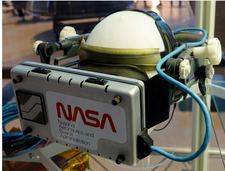
Fig. 2.17. One of the first VR headset (1985), made by Jim Humphries and Mike McGreevy at NASA's Ames Research Center in California. The system created a computer-generated image of what a pilot might see during an actual flight. It was intended to test concepts of presenting visual information to pilots or astronauts. Sensors tracked the movement of the wearer's head, and the displayed images moved accordingly. James Humphries donated this to the Museum in 1997. Picture taken at the National Air and Space Museum's Steven F. Udvar-Hazy Center in Chantilly, Virginia, USA. Author: Sanjay Acharya Source: Wikimedia commons, License: CC-BY-SA 4.0.
