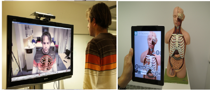
Fig. 2.6. Left: Magic mirror is an augmented reality system displaying augmented content on the user's body for educational purpose [30] ©2012 IEEE Right: The image shows another example of medical AR application where 3D model is augmented with informative text for educational purpose. Author: zedinteractive, Source: Wikimedia commons, License: CC0
