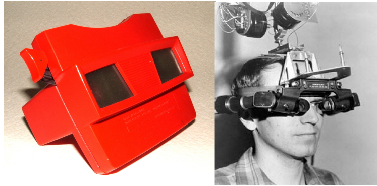
Fig. 2.8. (left) A view-master model G, introduced in 1962. It is a special type of stereoscope where two images are displayed simultaneously using transparent color film. Author: ThePassenger, Source: Wikimedia commons, License: CC-BY-SA 3.0. (right) Ivan Sutherland wearing the head mounted augmented reality display. © Ivan Sutherland, reprinted with permission.
