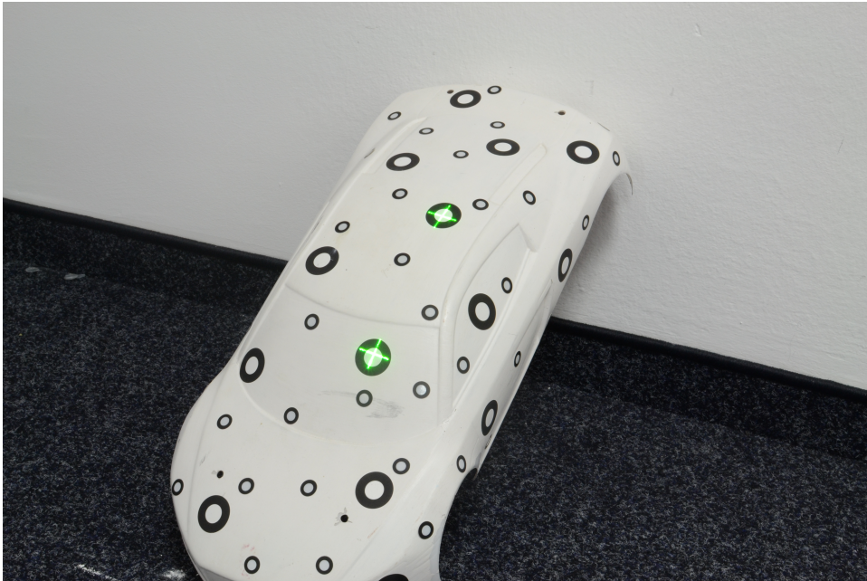
Fig. 3.12. The image displays a mock car model with several uncoded markers. The position of these markers are computed using optical measurement systems. The image displays a laser pointer projected at two different markers. This is one example use case of our SAR device. The measurements are directly presented on the part which makes decision making more intuitive. The image is part of test dataset Image ©Extend3D GmbH, published with permission.
