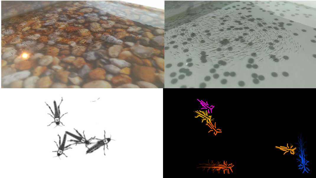
Fig. 5.5. (top) Mixed-Reality with multiple animals : A school of fish in a large fish tank where bottom of the tank is illuminated with multiple projectors to provide desired visual stimulus to a group, (bottom) Tracking multiple animals : Locusts with markers and 2D posture tracking of locusts using DeepPoseKit [82]
