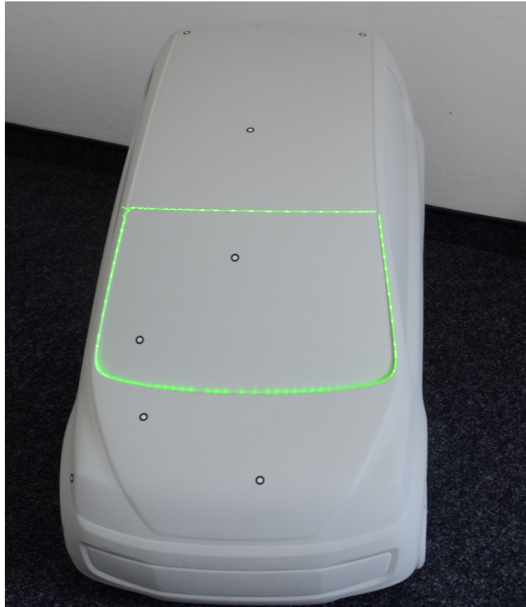
Fig. 4.4. A car model with example projection on the wind shield. The model is covered with uncoded markers used in metrology. ©2016 IEEE [148]
