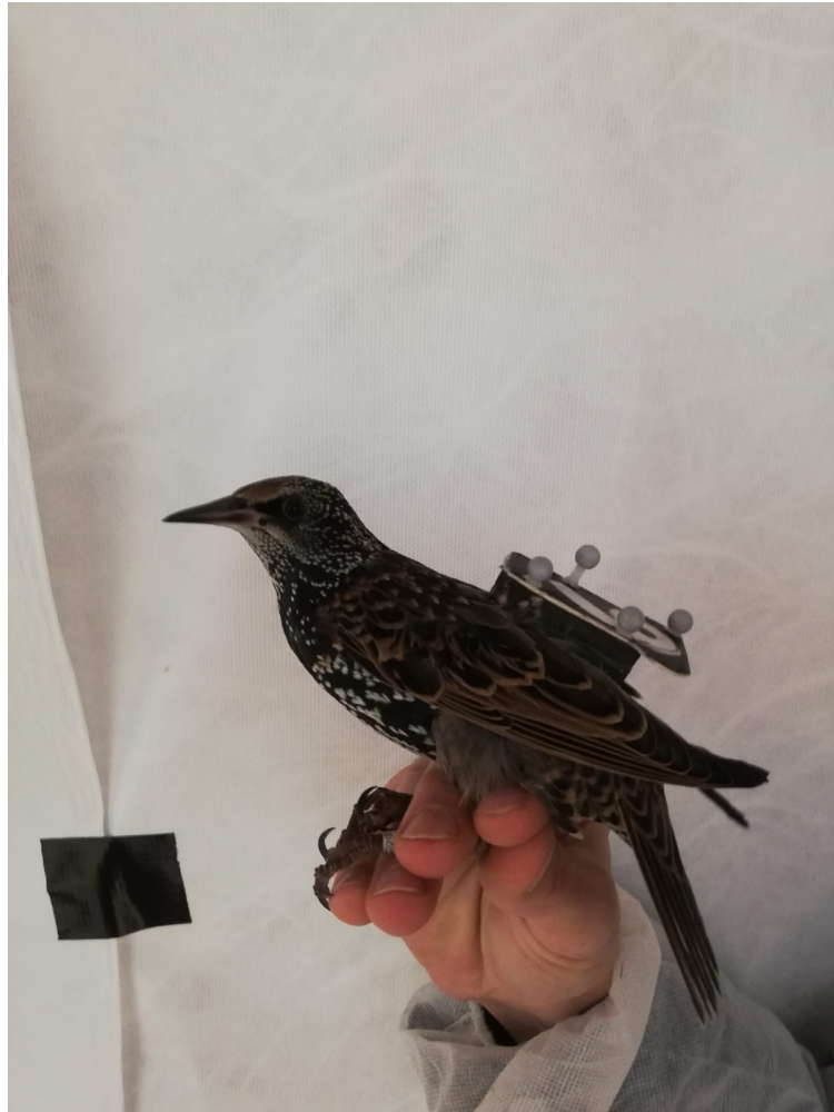
Fig. 6.4. The image shows a starling with a custom-designed backpack. The backpack has 4 markers of 6 mm size arranged in a unique pattern. It should be noted that the system can handle both 2D and 3D patterns, therefore the 3D pattern is achieved by raising the height of one of the markers. The base is made of special material to keep the backpack lightweight. The backpack is placed on a slightly raised platform to avoid occlusion of markers while flying. The markers attached close to the back of birds may show irregular tracking patterns because the line of sight is broken with one or more cameras. The image is part of a study conducted by Nora Carlson to understand the collective behavior of starlings ©Nora Carlson.
