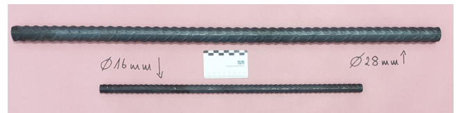
FIGURE 2 Rebar specimens for fatigue testing
