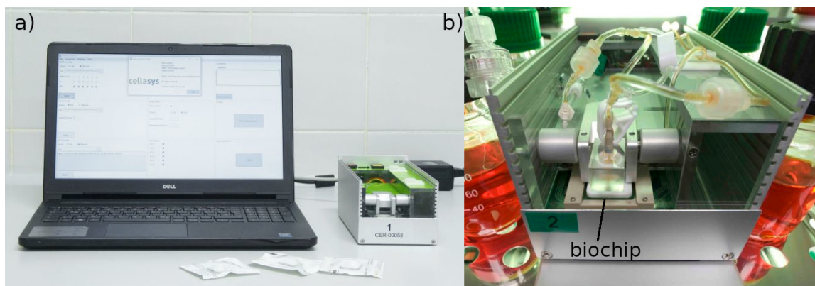
Figure 2.4: Intelligent Mobile Lab (IMOLA): a) shows the IMOLA on the right with a Laptop in the left that is used for data recording and display. b) shows the IMOLA in detail. The inserted biochip is labelled. It is held in place by a fixture. The micro-fluidic connectors and tubing are also visible. Next to the IMOLA there are several flasks with cell culture media being pumped through the chip. Adapted from cellasys' website [37], rearranged and subfigure designators added. Reproduced with permission from cellasys GmbH.
