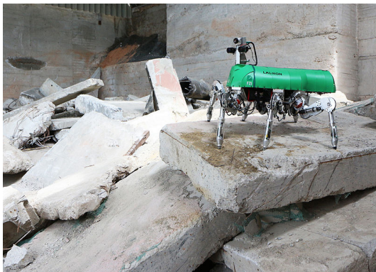
(a) Lauron V developed by FZI suitable for Search & Rescue applications. [1]
