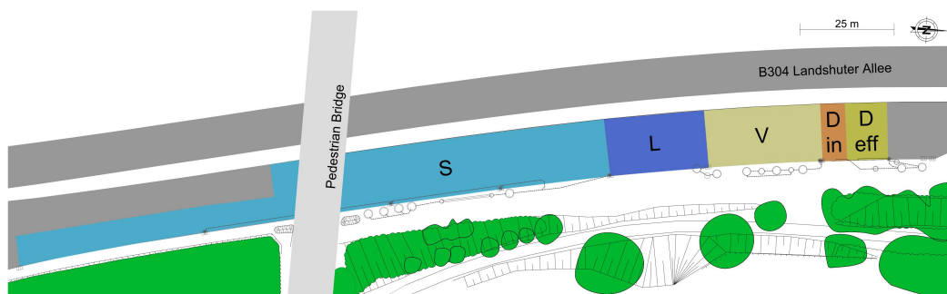
Fig. 3.1. Layout of the monitoring site in Munich, Germany. The different colors (except for green) indicate the catchments of the individual SQIDs. S was the SediSubstrator XL 600/12, Fränkische Rohrwerke; L was the individually designed SQID for the City of Munich; V was the ViaPlus 500 with upstream sedimentation shaft, Mall; D was the Drainfix Clean 300, Hauraton; D in indicates the catchment were influent samples of D were withdrawn and D eff the catchment of SQID D. Source of the layout: City of Munich.
