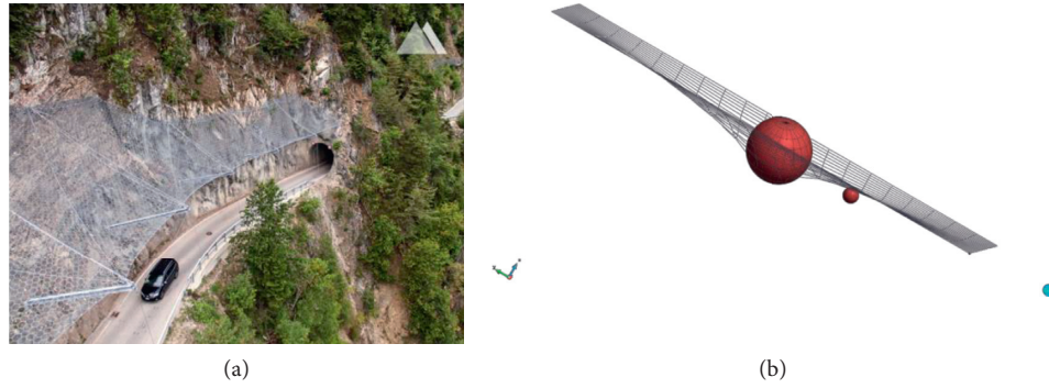
FIGURE 18: Picture of protection net and corresponding numerical model, including the net as cable structure and two impacting rocks modelled as single DEM particles. The one particle is chosen to be so small that it falls through the net, to verify the correct coupling detection. (a) Route Chalais-Vercorin, Valais [45]. (b) Numerical DEM-FEM coupled model.
