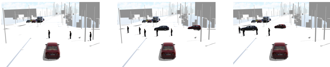
Figure 11. 3D visualization of the simulation scenario at runtime, whereby the vehicles are inserted by VTD and the static object geometries were generated from CityGML before runtime.
