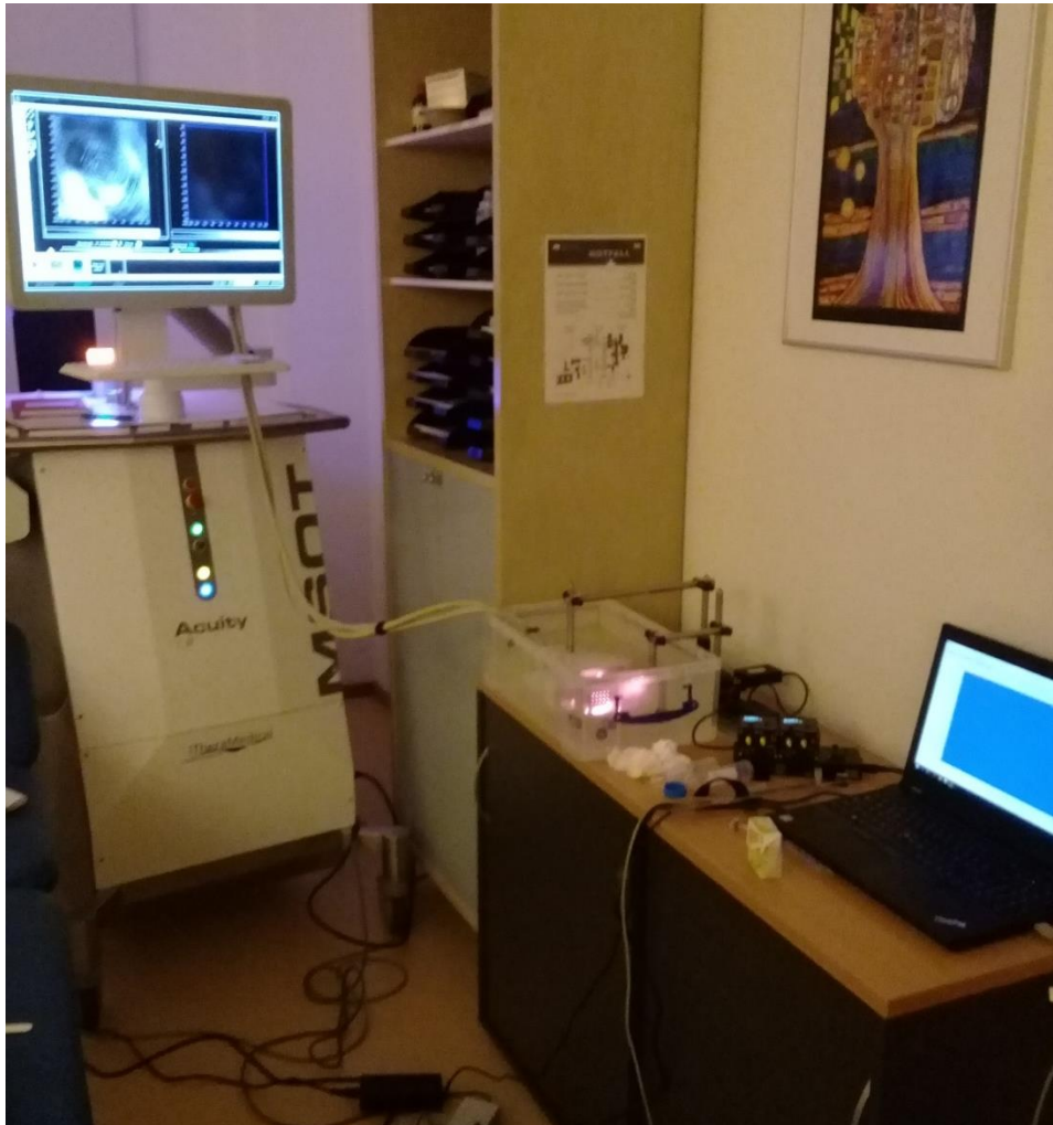
Figure 4.7: The handheld optoacoustic imaging system. Photograph showing the MSOT Acuity optoacoustic platform from iThera Medical GmbH and the handheld probe being characterized in water bath, using external motorized linear translation stages.
