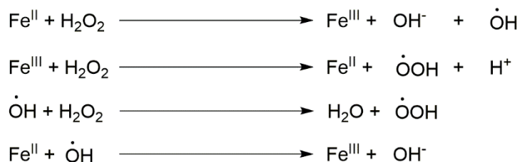
Scheme 2 Fenton-type reaction of hydrogen peroxide in the presence of iron cations. 82
