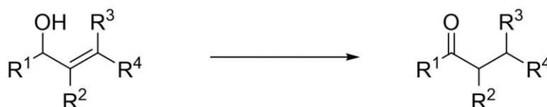
Scheme 4: Possibilities for the isomerization of allylic alcohols towards saturated ketones. The two-step isomerization involves two consecutive steps of oxidation and reduction respectively, while the one-step isomerization proceeds in a concerted fashion as alkene isomerization.
