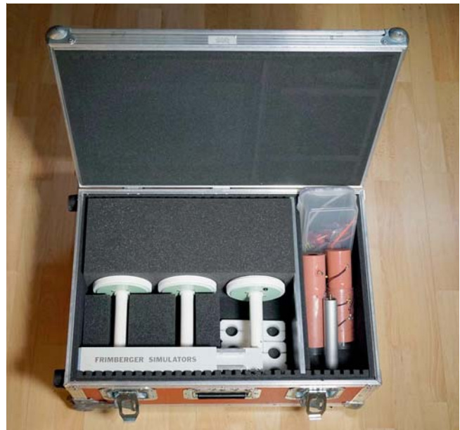
► Fig. 2 Transport case packed with three simulators, MSPS/HFPS, plus accessories. Please take note the extraordinarily small size of the simulators, which facilitates packaging and transport.
