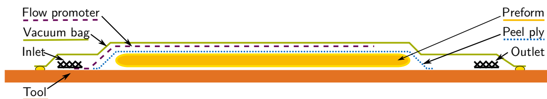
Fig. 3-3 Infiltration set-up used. The vacuum applied to the outlet sucks in the resin that is kept at ambient pressure. The resin flows from the inlet through the flow promoter into the dry preform.
