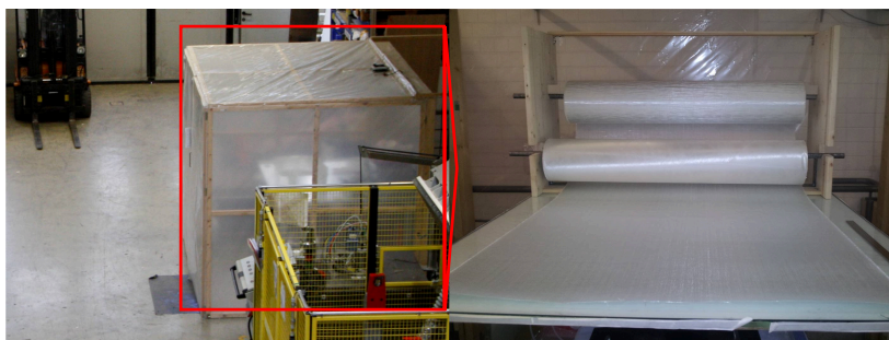
Fig. 3-2 Carbon fiber-free environment used for preforming of GFRP test plates and tools.
