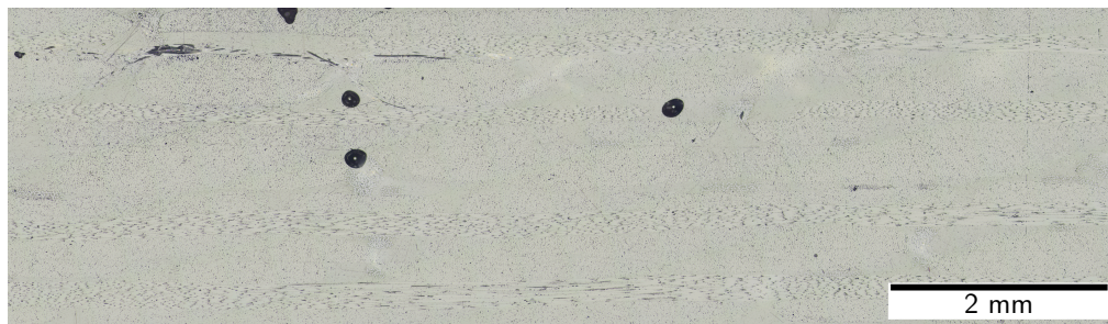
Fig. 3-15 GFRP microsection showing exemplary voids.
