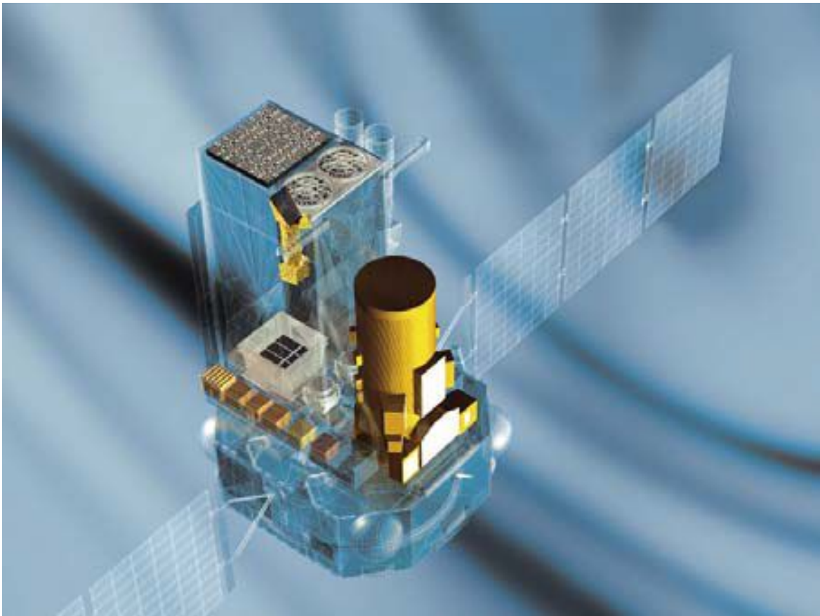
Figure 3.6: INTEGRAL spacecraft with lined out instruments. The spacecraft weighed 4 t at launch including 2 t of payload. Dimensions of the satellite are (5 \times 2.8 \times 3.2) \text{ m}^3 . The solar panel span a width of 16 m when deployed. Image taken from Schanne (2006).
