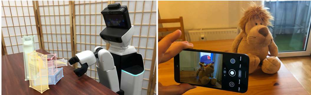
Figure 1.1. Exemplary Applications of 6D Pose Estimation. Left: The Toyota HSR robot is grasping the object of interest leveraging the estimated 6D object pose [10][©2019 IEEE]. Right: Coherent augmentations are applied to the lion object using the inferred 6D pose information.
