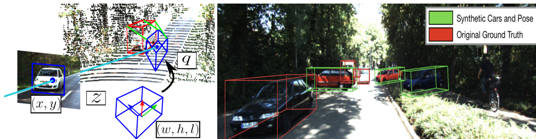
Figure 5.5. Lifting 2D Objects to 6D Pose and Metric Scale. Left: After lifting our 2D detections to 6D pose and metric scale, we instantiate the associated 3D bounding box and directly compare it against the associated groundtruth box. This avoids common pitfalls due to weighting different loss terms and directly optimizes for the desired goal, the best alignment in 3D. Right: After learning a shape space of cars using a 3D Convolutional AutoEncoder, we autolabel all images from the KITTI3D dataset and leverage the annotations for coherent synthesis of new training images.
