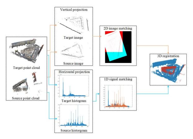
Figure 3.2: Workflow of the PBPC method.
