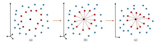
Figure 2.3: Illustration of LML methods. a) Neighborhood recovery, b) computation of affinity weight, c) calculation of embedding.
