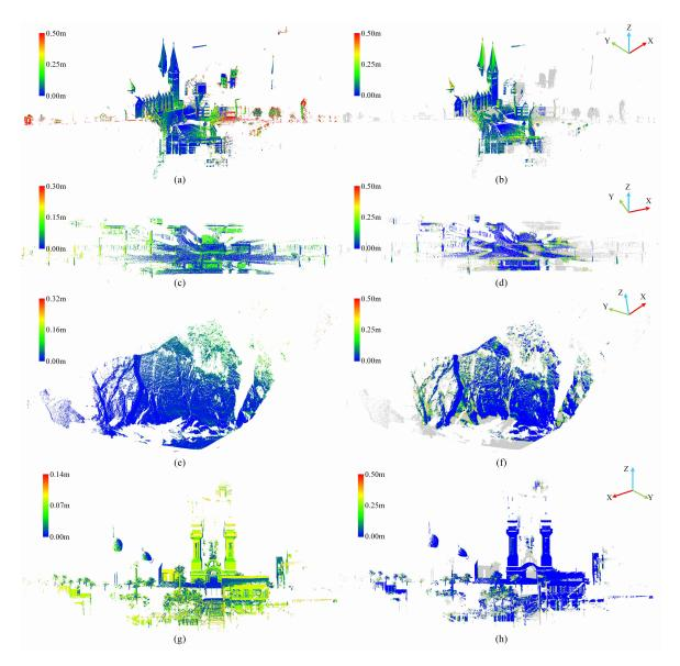
Figure 7.8: Selected registered results colored by the residual distances between corresponding points, where the gray points represent the non-overlap areas. Point distances between ground truth and the align source scan in a) Bremen, c) WHU-TLS subway, e) WHU-TLS mountain, and g) Resso. Point distances between target and the aligned source scans in b) Bremen, d) WHU-TLS subway, f) WHU-TLS mountain, and h) Resso.
