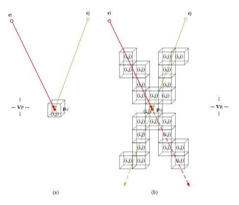
Figure 5.3: Storage of camera indices in 3D grids. a) Rays from two camera positions  $\mathbf{c}_i$  and  $\mathbf{c}_j$  intersect in position  $\mathbf{p}_{i,j}$  located in the 3D grid cell  $\mathbf{V}_P$ . Corresponding camera indices are stored in the cell, b) rays from camera positions  $\mathbf{c}_i$  and  $\mathbf{c}_j$  traverse 3D grid cells  $\mathbf{V}_R$ . The same indices are stored in the traversed grid cells.
