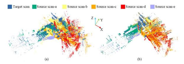
Figure 7.5: Registration results of the Resso dataset using GRPC, with color representing different scans. (a) Source and target point clouds shown in the same coordinate frame. (b) Aligned source and target point clouds.
