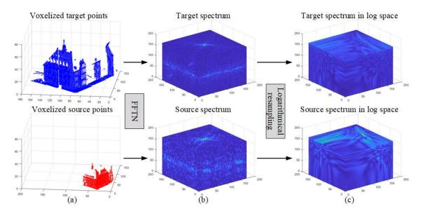
Figure 3.15: Scaling estimation using FMT. a) Discrete 3D signals, b) spectrum of discrete 3D signals, c) Spectrum in log space after FMT.
