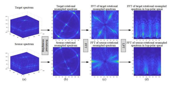
Figure 3.13: Illustration rotational resampling. a) Spectrums from 3D signals, b) rotational resampled spectrum, c) FFT of rotational resampled spectrum, d) FFT of rotational resampled spectrum in log-polar space.
