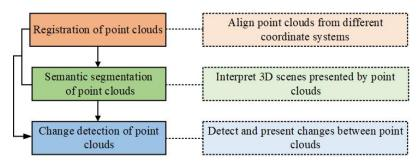
Figure 1.2: Three-step workflow for change detection from point clouds.
