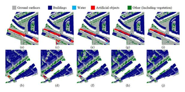
Figure 7.19: Details of the classification results with the AHN3 dataset for comparison. a) - b) Ground truth of test areas, c) - d) classification results with SDF, e) - f) classification results with MDF, g) - h) classification results with JME, i) - j) the smoothed classification results.
