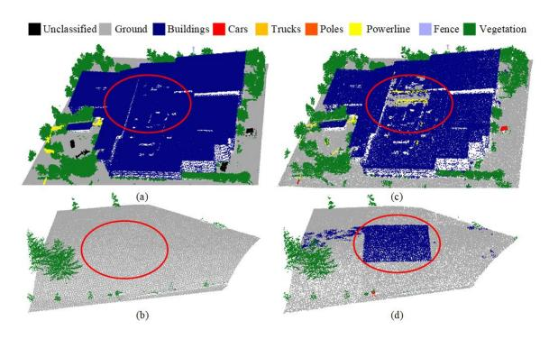
Figure 7.28: Details of classification results of the DALES dataset using GraNet. Only two selected examples are shown. a) - b) ground truth, c) - d) GraNet.
