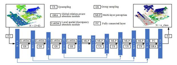
Figure 4.11: Detailed network architecture of GraNet.
