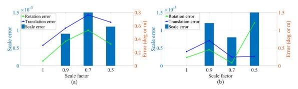
Figure 7.10: Sensitivity analysis of GRPC on changes of scale. a) Results using Resso dataset, b) results using WHU-TLS mountain dataset.
