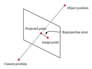
Figure 2.12: Illustration of reprojection error.
