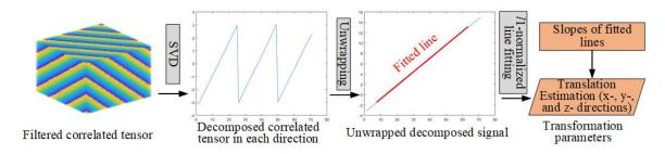
Figure 3.11: Illustration of the robust estimation of 3D shifts using  $\ell 1$  norm.
