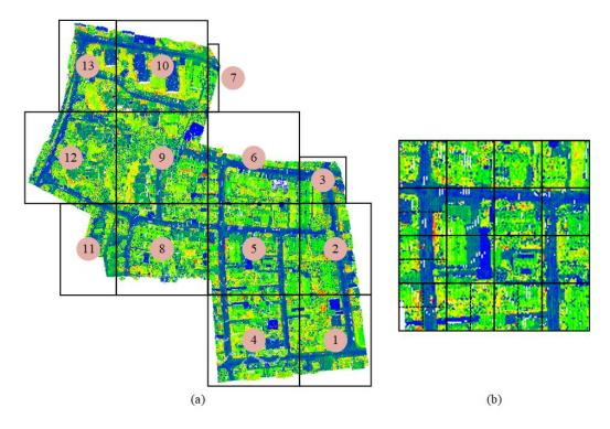
Figure 6.6: Illustration of the data division of the ISPRS benchmark dataset. a) The division of the large training blocks, b) the further subdivision of each training block.
