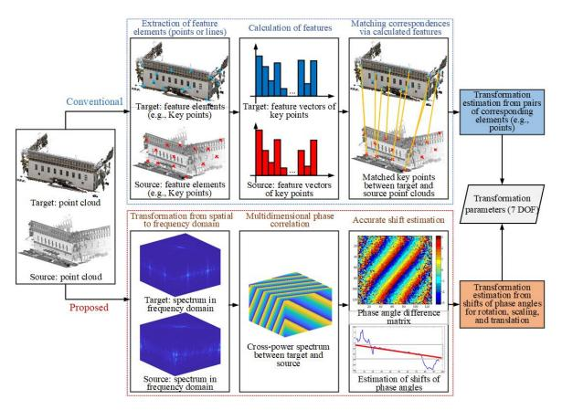
Figure 3.7: Workflow comparison of GRPC and conventional feature description-based strategy. Blue denotes the target point cloud. Red denotes the source point cloud.
