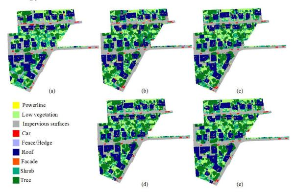
Figure 7.16: Classification results of test area 2. a) Ground truth, b) the classification result with SDF, c) the classification result with MDF, d) the classification result with JME, e) the smoothed classification result with GGO.
