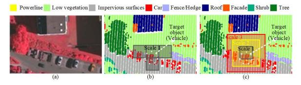
Figure 4.4: Reason for adopting hierarchical subdivision strategy. a) An illustration of the real scene as true orthophoto, b) the target vehicle is cut into pieces by the single-scale subdivision with fixed template size, c) the target vehicle can be fully represented by multiscale sub-pointsets in different template sizes. Labels are used for better illustration.
