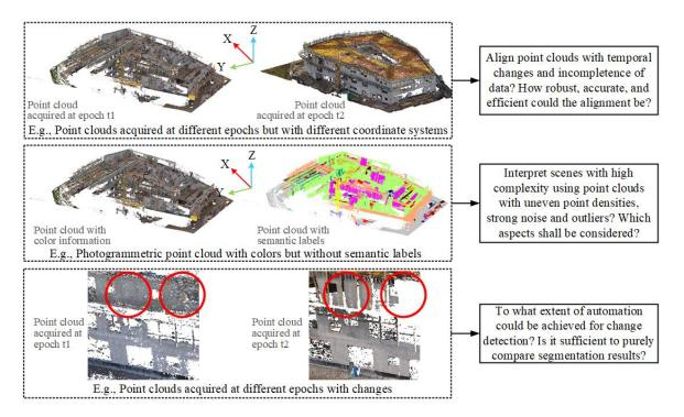
Figure 1.3: Problems for construction monitoring and change detection.
