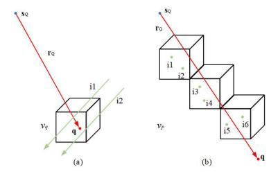
Figure 2.10: Conflicts between reference data (green) and the current measurement  $\mathbf{q} = \mathbf{s}_Q + \mathbf{r}_Q$  (red) : a) empty space at  $\mathbf{q}$  and b) occupied space along  $\mathbf{r}_Q$  [Hebel, 2012].
