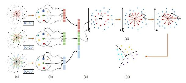
Figure 4.2: Workflow of the MLCE point cloud classification strategy. a) Scaling, b) geometric space, c) concatenation, d) embedding, e) classification.
