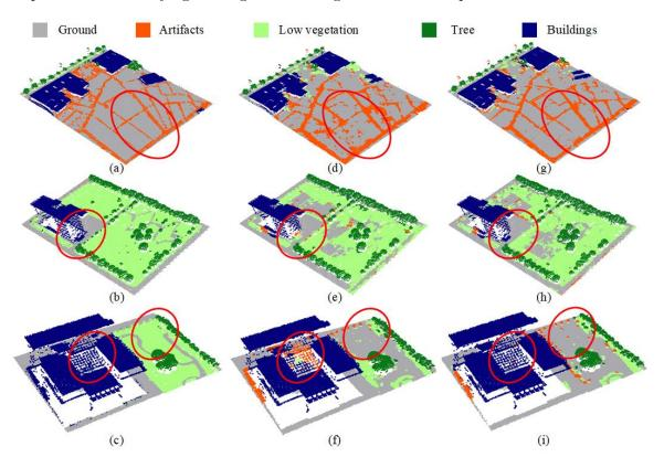
Figure 7.26: Details of classification results of the LASDU dataset using GraNet. a) - c) Ground truth, d) - f) PointSIFT, c) - i) GraNet.
