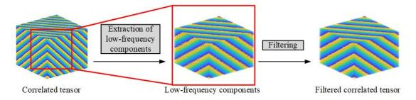
Figure 3.10: Illustration of extraction of low-frequency components.
