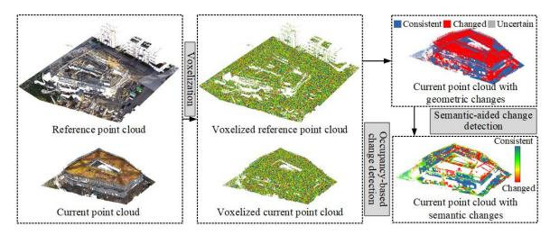
Figure 5.2: Workflow of change detection procedure.
