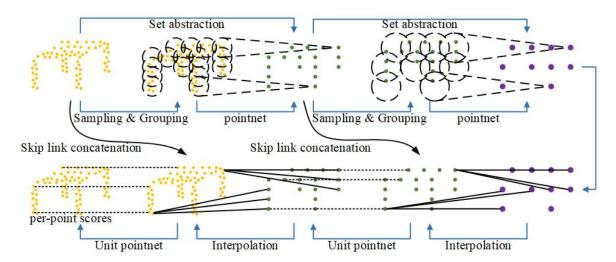
Figure 2.4: Illustration of the hierarchical architecture of PointNet++.
