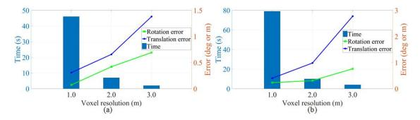
Figure 7.9: Sensitivity analysis of GRPC on voxel resolutions. a) Results using the Resso dataset, b) results using the WHU-TLS mountain dataset.
