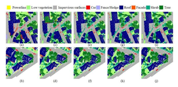
Figure 7.17: Details of classification results of the ISPRS benchmark dataset for comparison. a) - b) Ground truth, c) - d) the classification result with SDF, e) - f) the classification result with MDF, g) - h) the classification result with JME, i) - j) the smoothed classification result with GGO.
