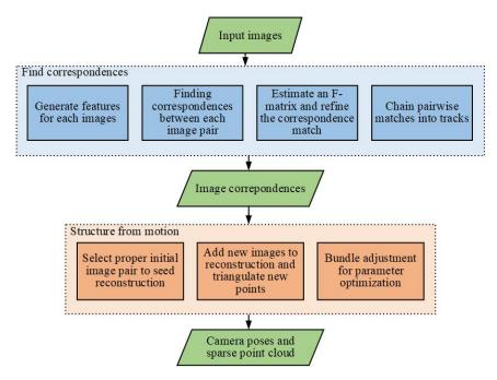
Figure 2.11: The process of SfM.
