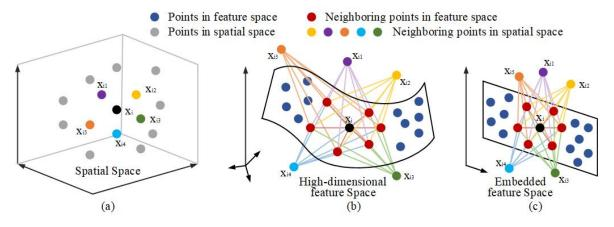
Figure 4.6: Integration of spatial information in joint embedding. a) Recovery of the spatial neighborhood, b) computation of reconstruction weight with the spatial constraint, c) calculation of joint embedding.
