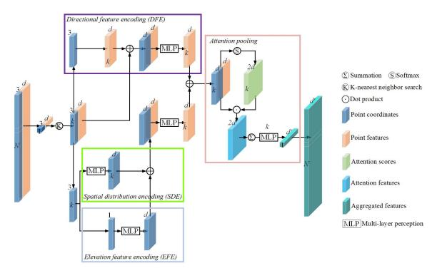
Figure 4.8: Exploited local spatial discrepancy attention encoding module. The purple panel shows the directional feature encoding module. The pink panel shows the attention pooling module. The light green panel shows the spatial distribution encoding module and the blue one shows the elevation feature encoding module.
