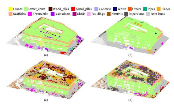
Figure 7.30: Semantic segmentation results of the construction dataset. a) - b) Ground truth, c) - d) the semantic segmentation results of the construction dataset using GraNet.
