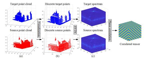
Figure 3.9: Multidimensional phase correlation. a) Original point clouds, b) voxelized 3D points, c) spectrum of discrete 3D signals after FFT, d) correlated tensor from phase correlation of spectrums.
