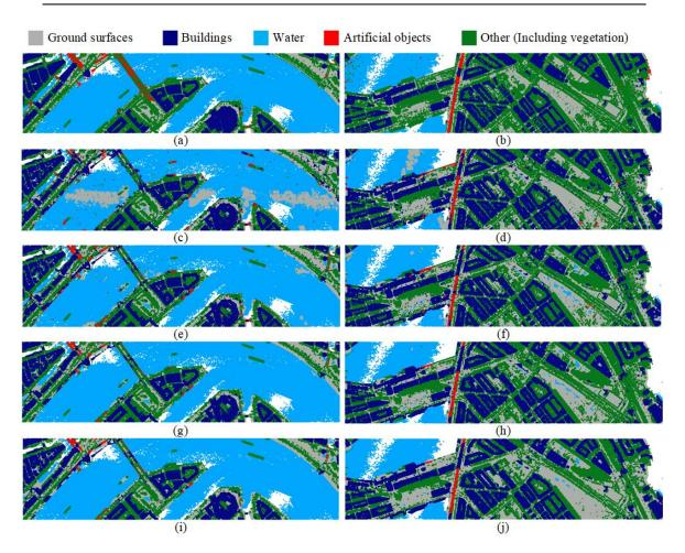
Figure 7.18: Classification results of the AHN3 dataset. a) - b) Ground truth of test areas, c) - d) classification results with SDF, e) - f) classification results with MDF, g) - h) classification results with JME, i) - j) the smoothed classification results.
