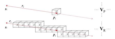
Figure 2.7: Filling of the voxel grids  $\mathbf{V}_P$  and  $\mathbf{V}_R$ . i: index;  $\mathbf{s}_i$ : sensor position;  $\mathbf{p}_i$ : laser point;  $\mathbf{r}_i$ : range measurement [Hebel et al., 2011].
