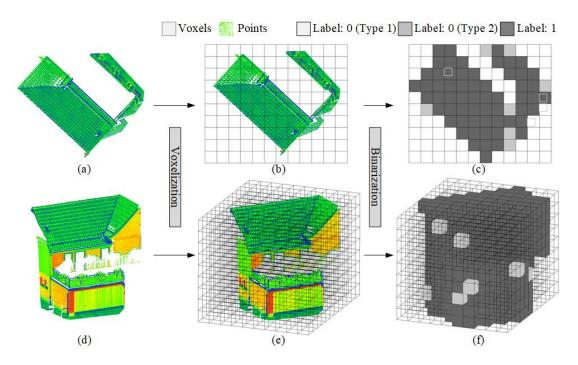
Figure 2.6: Voxelization and binarization of point clouds. a) Original point clouds from top view and d) from oblique view, b) voxelized point clouds from top view and e) from oblique view, c) binarized voxels from top view and f) from oblique view. It should be noted that Type 1 denotes the empty voxels annotated with value zero and Type 2 denotes the voxels with limited numbers of points and annotated with value zero.
