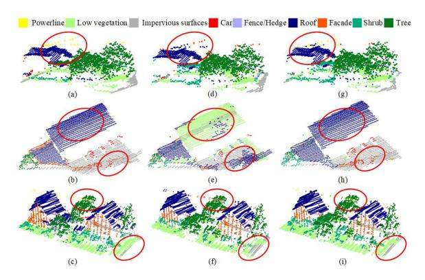
Figure 7.23: Details of classification results of the ISPRS benchmark dataset. a) - c) Ground truth, d) - f) PointSIFT, g) - i) GraNet.
