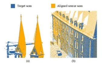
Figure 7.2: Details of the registration result of the Bremen dataset using GRPC. a) - b) Scene sections of the registered point clouds.
