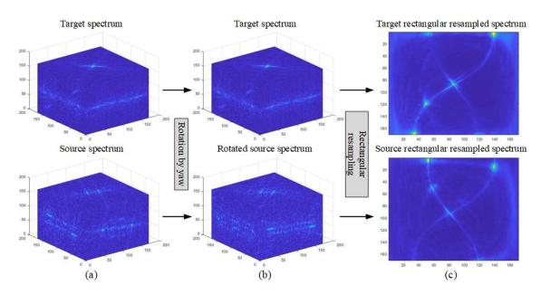
Figure 3.14: Illustration of rectangular resampling. a) Spectrums from 3D signals, b) target spectrum and rotated source spectrum, c) retangular resampled spectrum.
