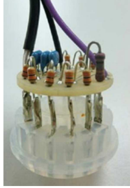
Figure 2.31: Photo of a voltage divider, from [169; p. 86]. Note the resistors and capacitors between the leads, which are plugged onto the pins emerging from the PMT stem.
