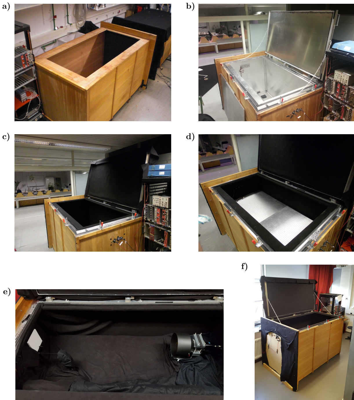
Figure 3.4: Shielded Photosensor Analysis eXperiment (SPAX): A photosensor characterization setup specialized on timing and small-charge effects which was developed and continuously improved during this work.
