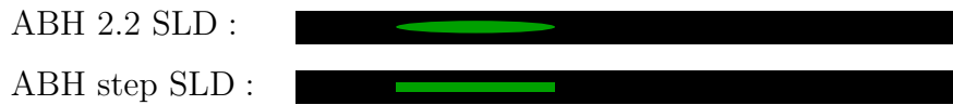
Figure 5.15: Two different thickness profiles that follow an integrated sandwich layer damping (SLD).
