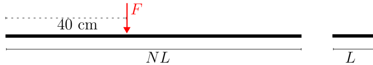
Figure 5.33: Model of a free-free beam that consists of ten identical unit cells of length L = 10 cm.
