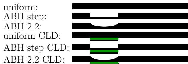
Figure 5.3: Labeling of the different thickness profiles made of titanium (black) and a damping material (green).
