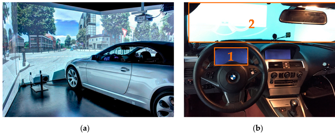
Figure 1. (a) Static driving simulator of the Chair of Ergonomics [32]; (b) driver's cockpit with the defined areas of interest (AOIs) instrument cluster (1) and windshield (2) marked orange.
