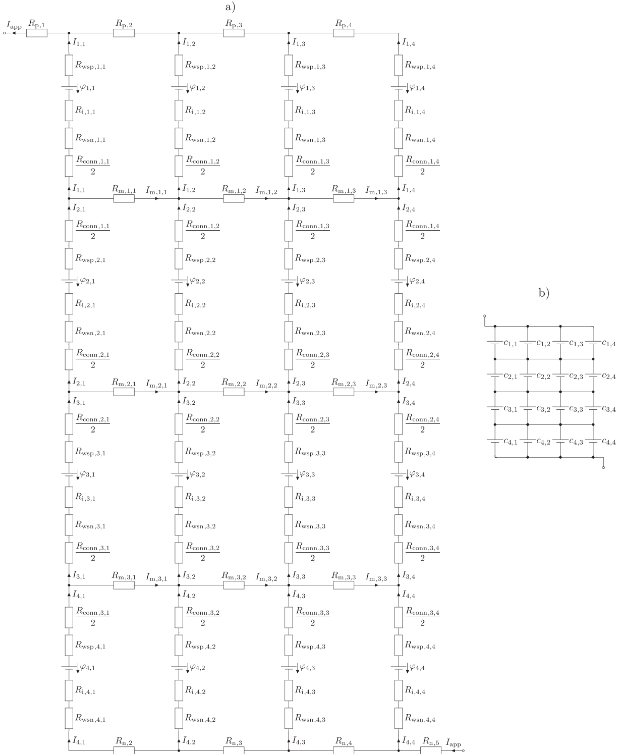
Figure 1. System topology of the ELM for a 4s4p system. Part (a) shows the entire system, including all of its components. Part (b) is the graphically reduced version and will be used instead of (a) in the following. For both versions, the STs are positioned in a cross wise manner. Cross-connectors between adjacent strings and cells resemble a connector plate.
