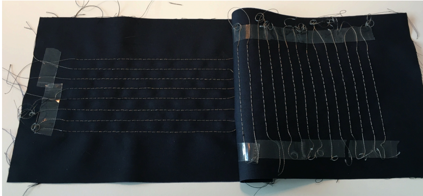
Figure D.3: Aligned fabric halves without piezoresistive layer. Fixing pins are used on the right edge of the two layers to keep the alignment.
