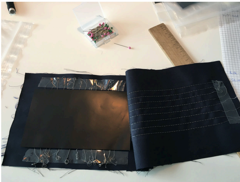
Figure D.4: Aligned fabric halves with piezoresistive layer.
