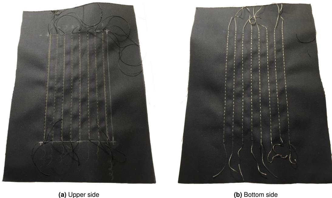
Figure D.2: One fabric half with sewed-in steel threads.
