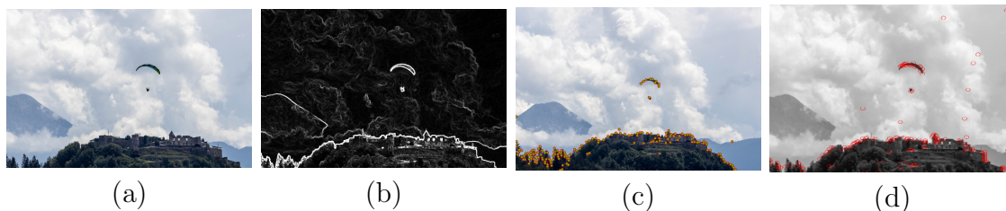
Figure 2.10: Feature extraction in camera imagery.
