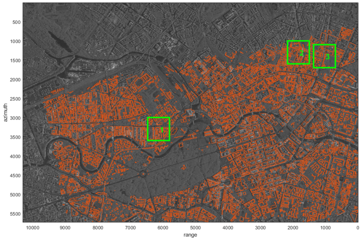
Figure 5.5: The study area in the SAR image coordinate system. GIS building footprints (red) are radar coded in the SAR image coordinate system with a constant height of 77.5 m. For detailed inspection of the two point-sets before and after registration, three small areas in the green rectangles are selected: Area 1, 2, and 3 represent areas where registration procedures are needed at global, subarea, and polygon levels, respectively. The point-sets in each area are shown in Figure 5.7.
