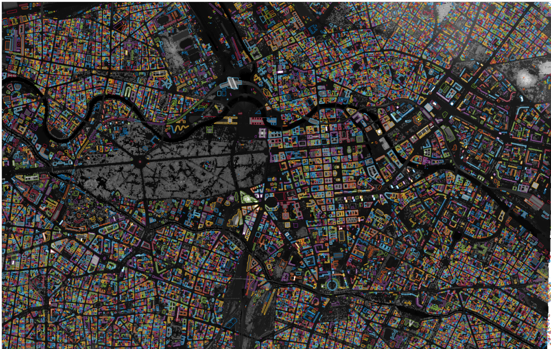
Figure 4.4: Building footprint polygons superimposed on a DSM in Berlin that used in the thesis.
