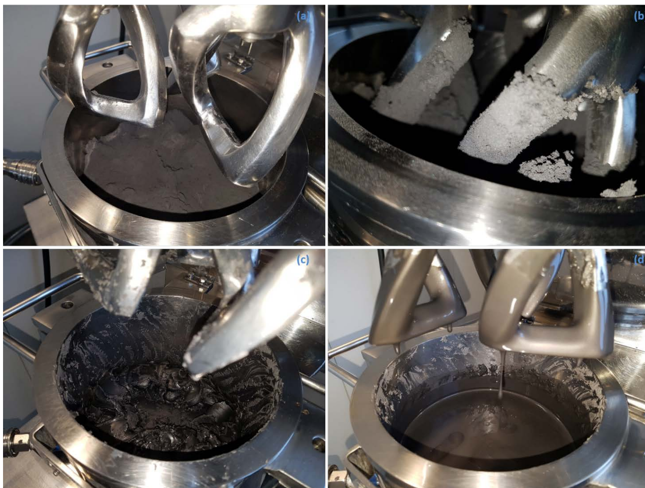
Fig. 2.5: Electrode slurry preparation using a kneader; (a/b) premixing phase; (c) kneading phase; (d) dilution phase.
