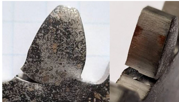
Fig. 10 Exemplary photograph of the occurred tooth root breakages
