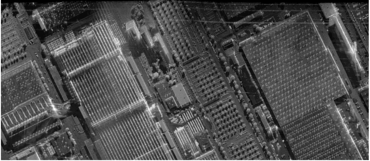
Figure 2.2: Ka-band SAR image acquired on a linear trajectory showing an industrial complex and several parking areas in Woerth, Germany. Resolution is 25 cm. More sensor and processing specifications are presented in [Palm et al., 2016c].
