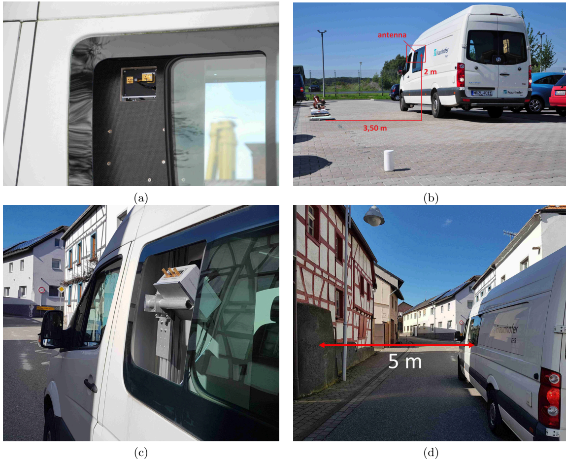
Figure 7.7: Carborne MRM experiments. a) Antennas behind the window in street mapping mode. The window is opened while operating, b) distances of an experimental setup in street mapping mode, c) antennas and front-end behind open window in facade mapping mode, d) geometry and distances in facade mapping mode.
