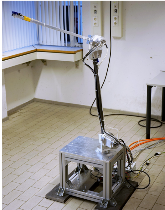
Figure 2.1: Modular, three-axis lightweight manipulator with structural elasticity 1
