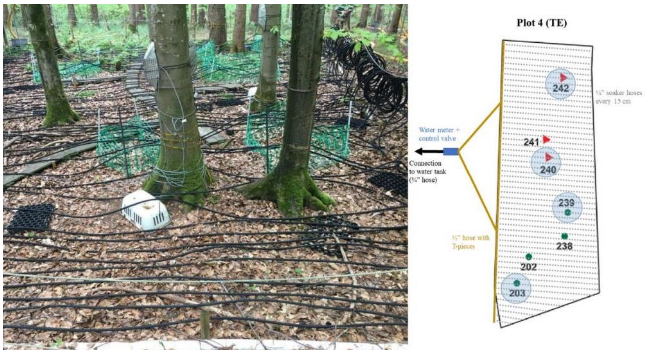
Figure 6: Example of the watering system on one CO plot (left) and schematic set-up of the watering system on plot 4 (right). (Altered from Article 1)
