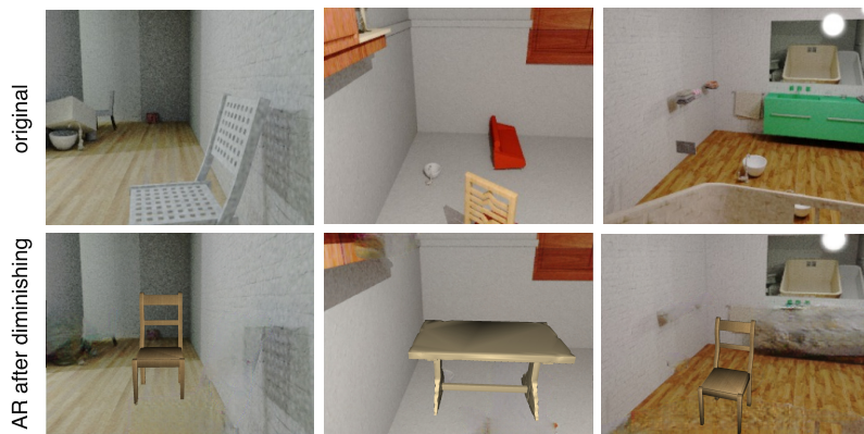
Figure 3.20. The proposed PBO method, applied to augmented-diminished reality. (Top) Input RGB image (Bottom) Result after background inpainting and rendering of new furniture.
