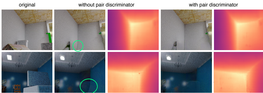
Figure 3.10. Qualitative results of the background completion RGB-D alignment. ( Left ) Original input. ( Center ) Result without pair discriminator. ( Right ) Result with pair discriminator.
