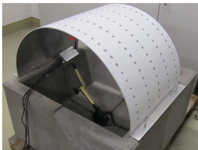
Figure 14. Set up of the demonstrator including a C-shaped aluminum sandwich panel mounted onto a concrete foundation. A modal hammer inside the foundation provides the excitation for the mobility measurements. The red cross approximately indicates the point of excitation on the inside of the panel.
