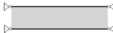
FIG. 2. Modeling of simply supported boundary conditions by constraining the displacement DOFs of the face sheet edges.
