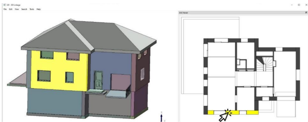
Figure 9.2 Linking 2D drawing to 3D model (Borrmann, Abualdenien, & Krijnen, 2021)
