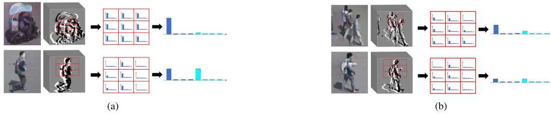
Fig. 8. Spatial motion characteristic embedded in single scale spatio-temporal feature for xy -plane (a) Abnormal events. Up: an activated event cuboid and its neighbour cuboids most locate within the contour of a fast moving object, their eHOFs will have larger magnitude on the motion direction, which results in the correspond average value of F_{xy} becoming large; Bottom: when activated event cuboid locate near the contour of fast moving objects, the eHOFs of neighbour cuboids inside contour will have larger magnitude on the moving direction, in contrast, the eHOFs of neighbour cuboids outside the contour, i.e. lie in background region or slow moving objects, will have small magnitudes, which results in the correspond variance becoming large. (b) Normal events. Either the mean or variance of normal events is smaller, no matter where the cuboids locate at.
