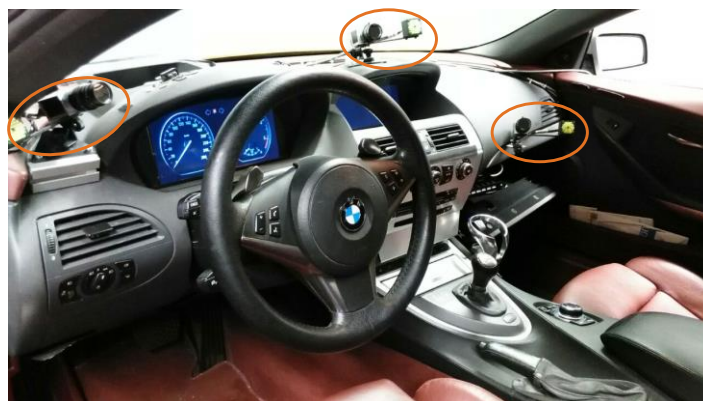
Figure 6-3. Position of the Smart Eye cameras in the interior of the driving simulator mock-up (Feierle, 2017).
