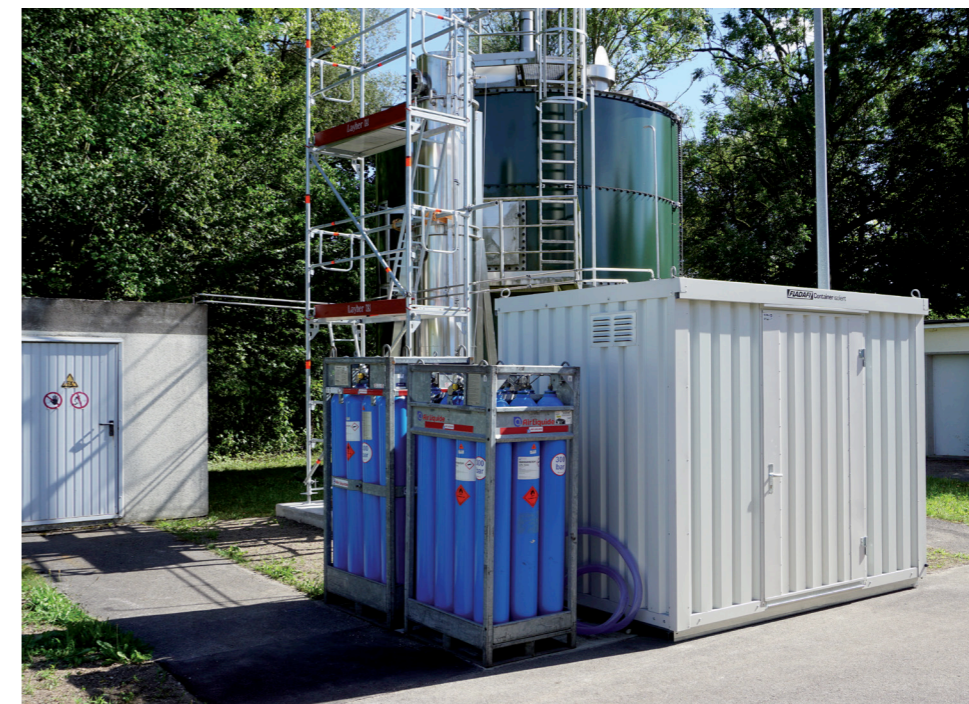
■ Pilot plant for methanation from waste water at the campus in Garching
