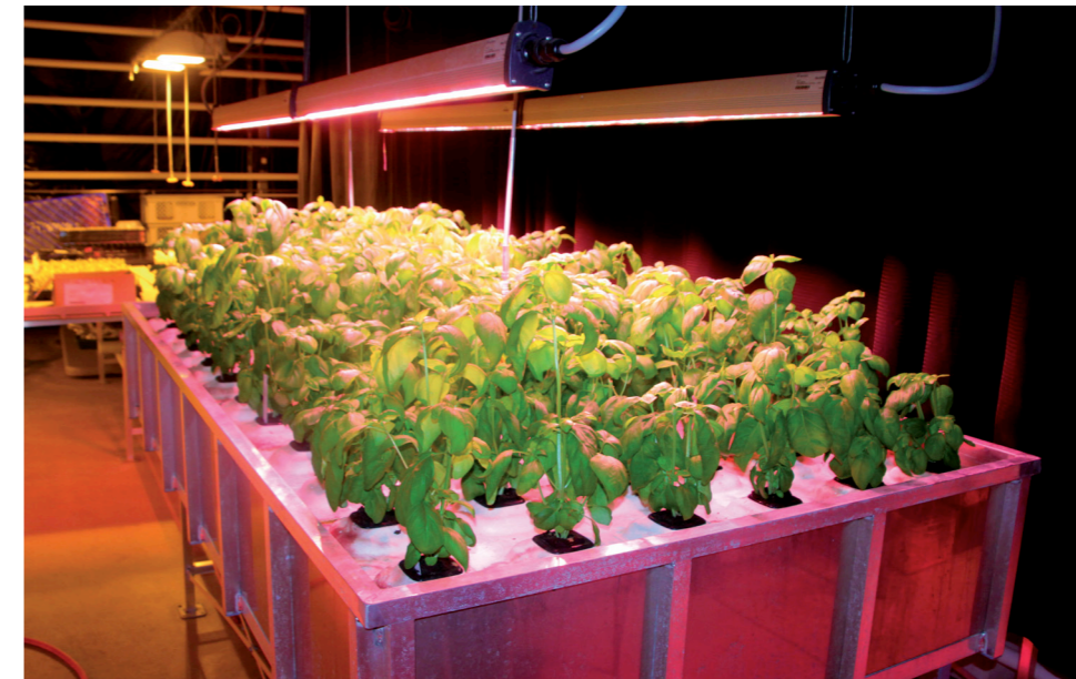
■ Fig. 10: Testing basil regarding the exposure to light: LEDs compared to sodium vapour lamps
