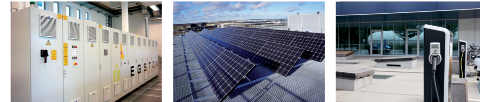
Fig. 3 Photos of the laboratory equipment. a) Egston load emulator; b) solar panels; c) EV charging stations
