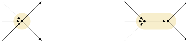
Figure 3.2: A reduction from directed vertex-disjoint paths to directed arc-disjoint paths. Every vertex of the original graph (left) is split into two vertices connected by a new arc (right). The incoming and outgoing arcs are separated by this splitting.
