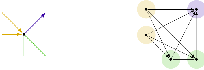
Figure 3.1: The construction of a line graph for mixed graphs. Every arc or edge in the original graph (left) is associated with a vertex in the line graph (right). Vertices representing two incident edges are connected by an edge. Vertices representing two incident arcs/edges which form a path are connected by an arc.
