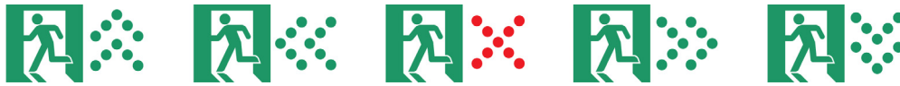
Fig. 1. Evacuation sign design. The four arrow designs were applied and animated with scrolling motion in both the non-adaptive and adaptive sign conditions. The blinking red “X” only appeared in the adaptive sign group.
