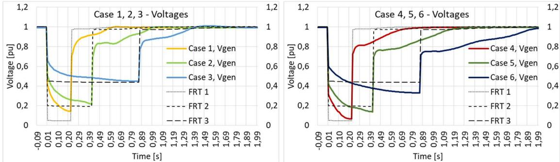
**Figure 3:** Comparison of voltage profiles between synchronous (left) and asynchronous (right) generators
