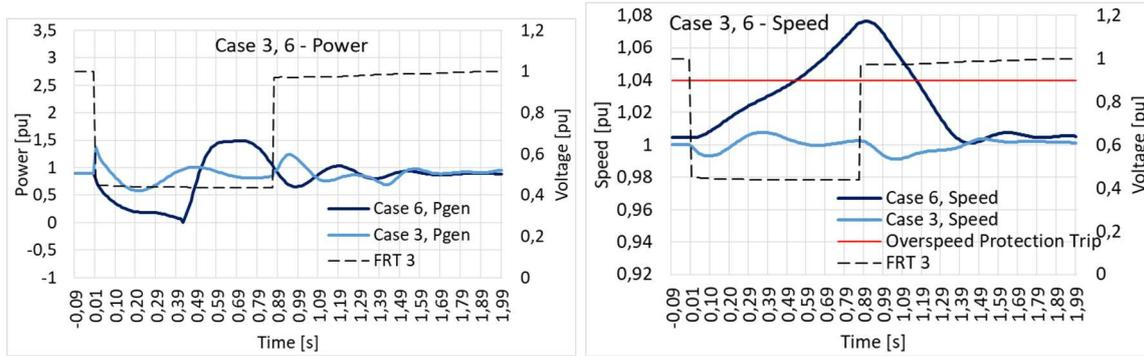
Figure 6: Comparison of power and overspeed between synchronous (case 3) and asynchronous (case 6) generators
