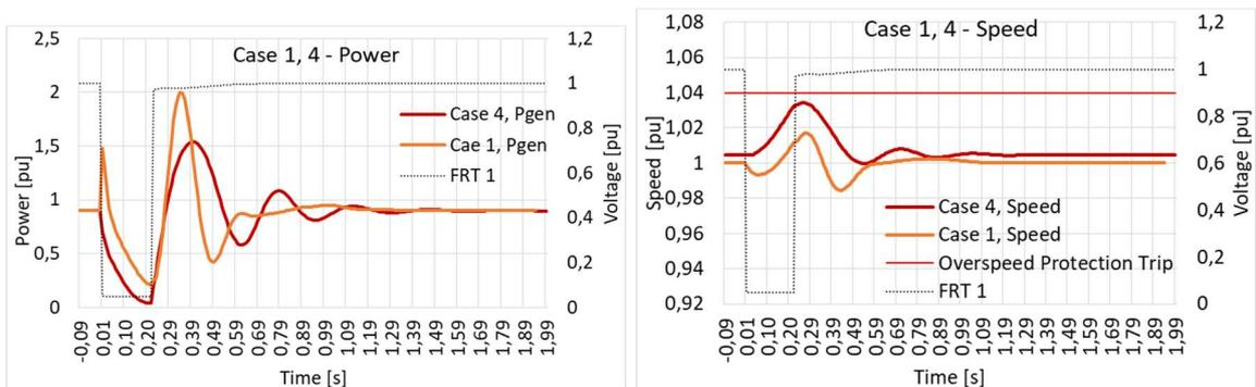
**Figure 5:** Comparison of power and overspeed between synchronous (case 1) and asynchronous (case 4) generators
