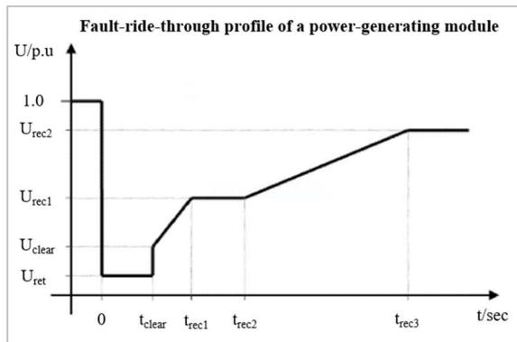
**Figure 1:** Fault-ride-through profile of a power-generating module according to RfG.
