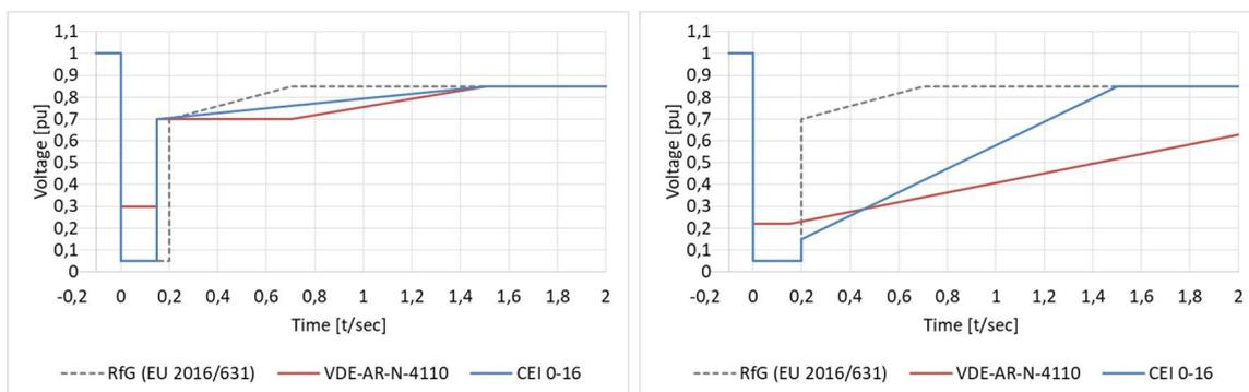
**Figure 2:** Fault-ride-through (FRT) limit curve for synchronous (on the left) and asynchronous (on the right) generators; comparison between RfG, German, Italian, English and French rules
