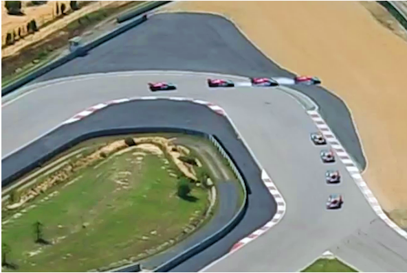
(a) Superimposed frames at 400 ms intervals taken from a video [290]. The lead vehicle exits the turn safely and the following vehicle leaves the track at the apex of the turn.
