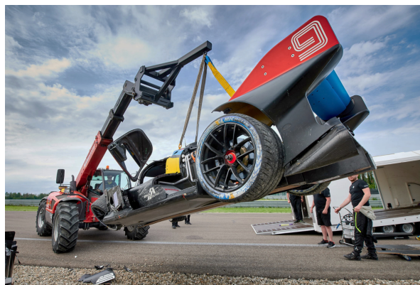
(b) Accident vehicle being recovered by track marshals and engineers using a telescopic forklift.
