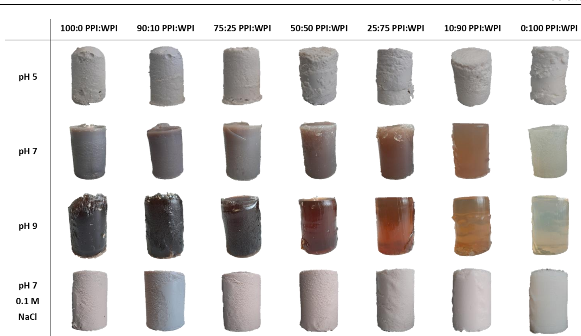
Figure 3-30 Optical appearance of protein solutions gelled for 15 min at 85 °C in dependence of pH and salt content as well as mixing ratio of WPI and PPI.
