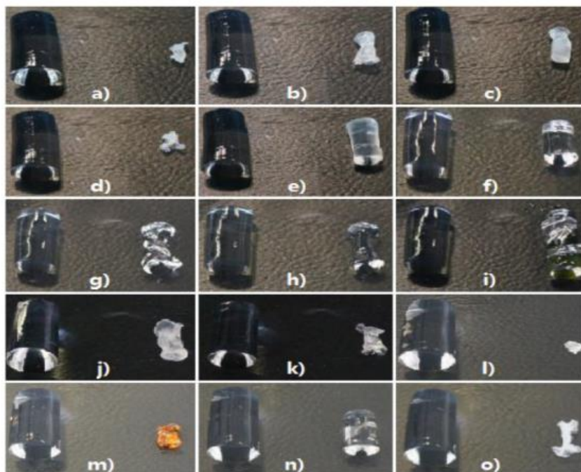
Figure 1-21 Shrinkage of alginate hydrogels in dependence of the solvent. (a) methyl ethyl ketone (MEK); (b) isopropanol (IPA); (c) acetone; (d) 1-butanol; (e) methanol (MeOH); (f) dimethyl sulfoxide (DMSO); (g) glycerol; (h) propylene glycol; (i) ethylene glycol; (j) ethanol; (k) 1,4-dioxane; (l) propylene carbonate; (m) furfuryl alcohol; (n) N,N-dimethylformamide (DMF) and (o) acetonitrile. Taken from Subrahmanyam et al., (2015)
