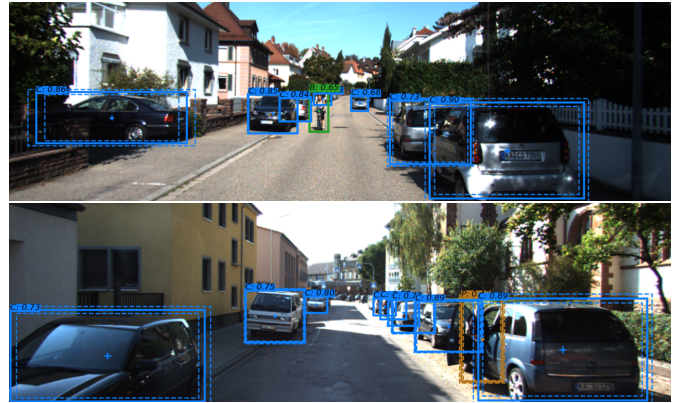
Fig. 1. Example predictions of the proposed CertainNet from the KITTI validation set [6]. Uncertainties for objectness, location and size are shown as the complement of the value at the top left of each box, the plus around the center, and dashed boxes respectively. The object class is color-coded.
