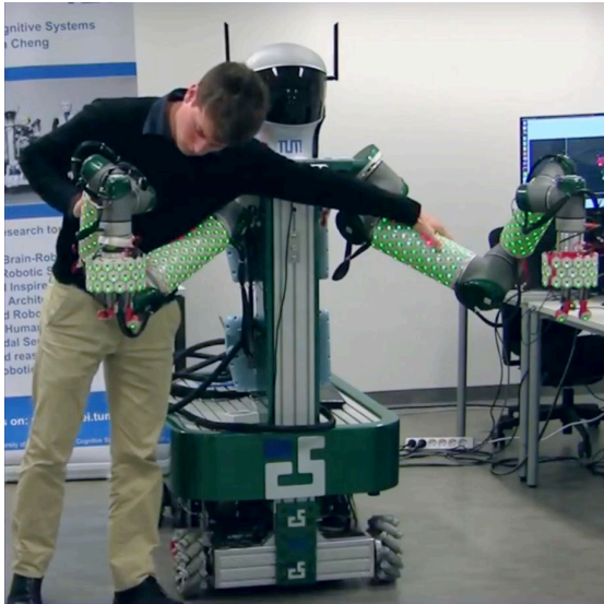
(iii) Multi-contact interaction with a dual-arm mobile robot covered with an artificial skin.
