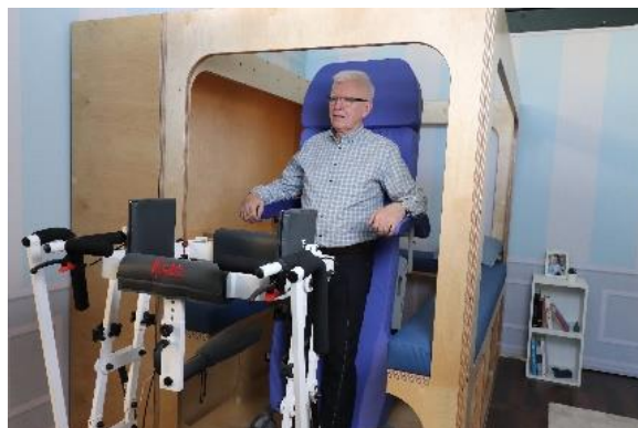
Figure 3-15: An older adult autonomously testing the SilverBed in three positions: lying, sitting, and standing
