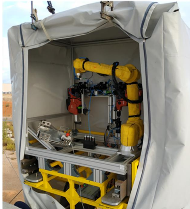
Figure 4-6: Robotic arm and its tools for bracket installation protected by weatherproof covers (photo: José David Jiménez-Vicaría).
