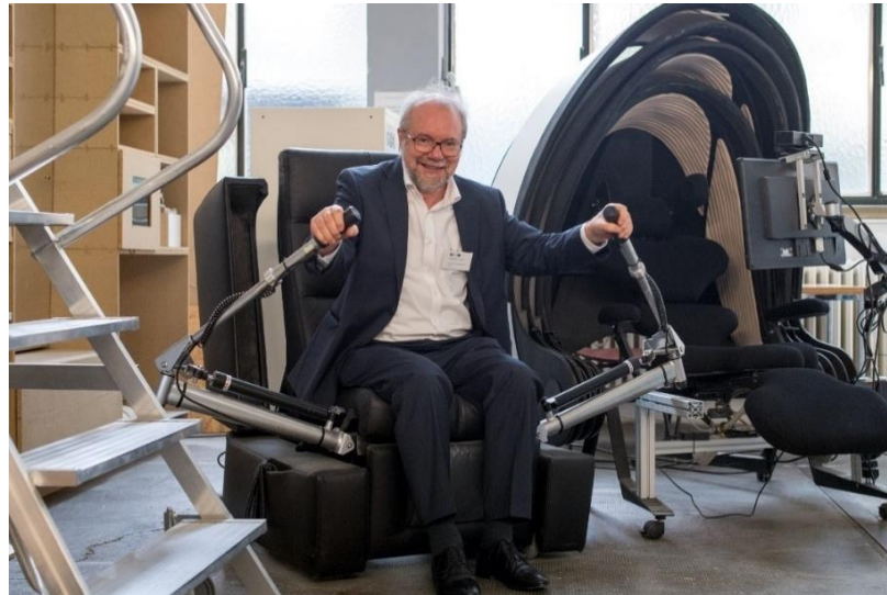
Figure 2-3: The GEWOS mechatronic chair with sensing and training features (Photo: T. Bock)
