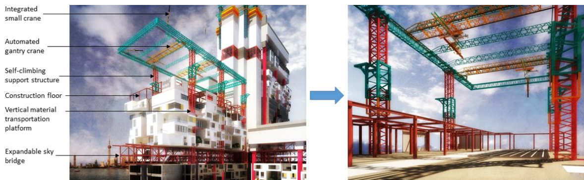
Figure 6-13: Exterior and interior views of the sky construction factory
