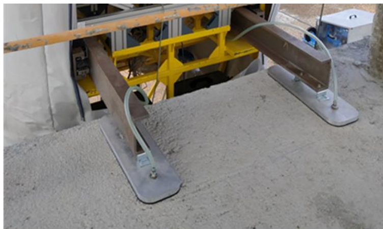
Figure 4-7: Stabilizer attaching the robot platform to the concrete slab (photo: José David Jiménez-Vicaría)
