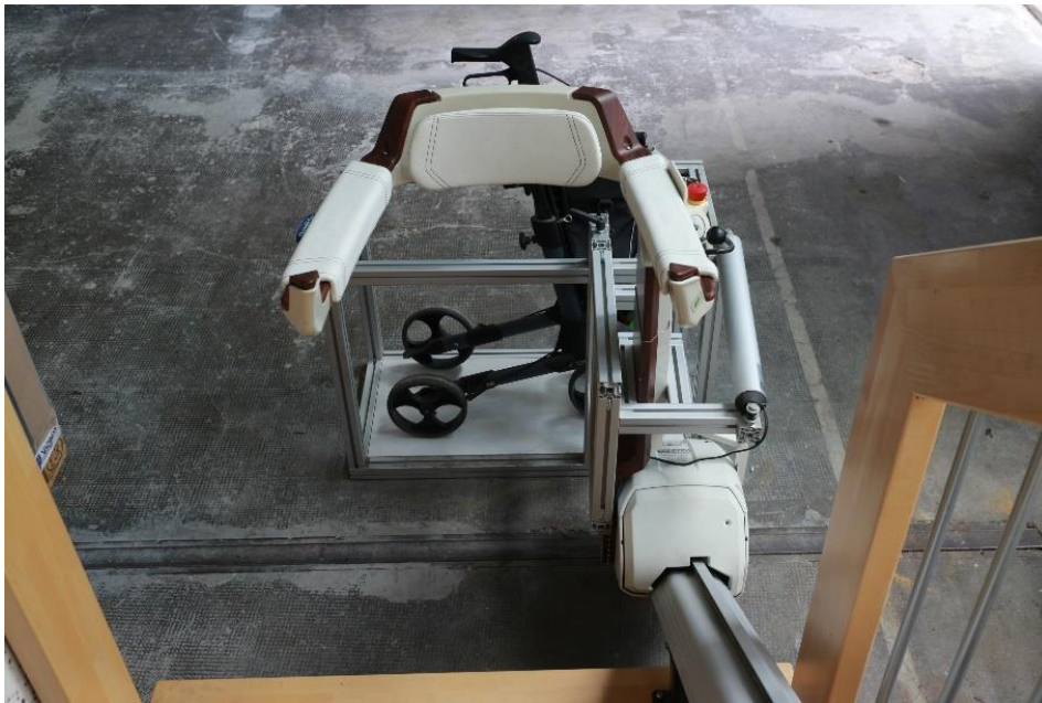
Figure 2-4: The StairWalker integrating a platform where the user put the rollator or grocery
