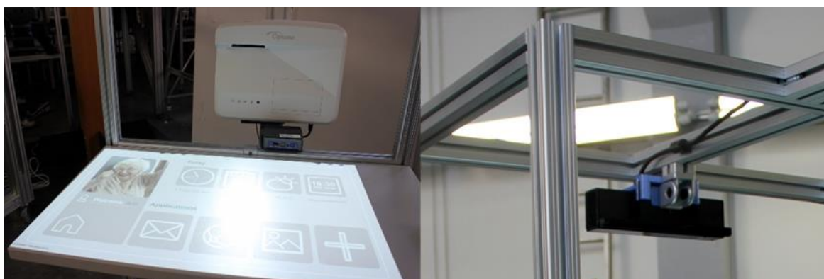
Figure 3-32: User interface and Kinect sensor in the MiniArc
