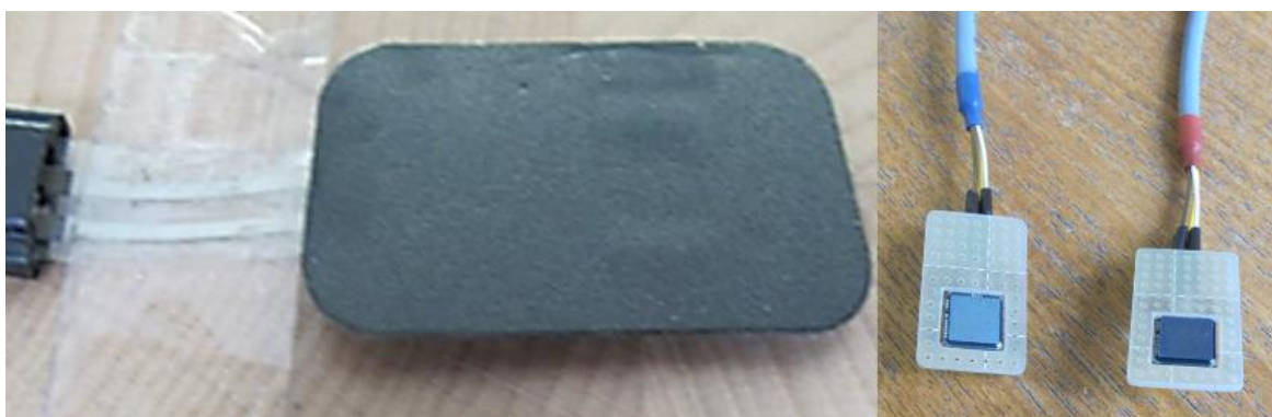
Figure 3-33: Activity monitoring sensors used in the iStander
