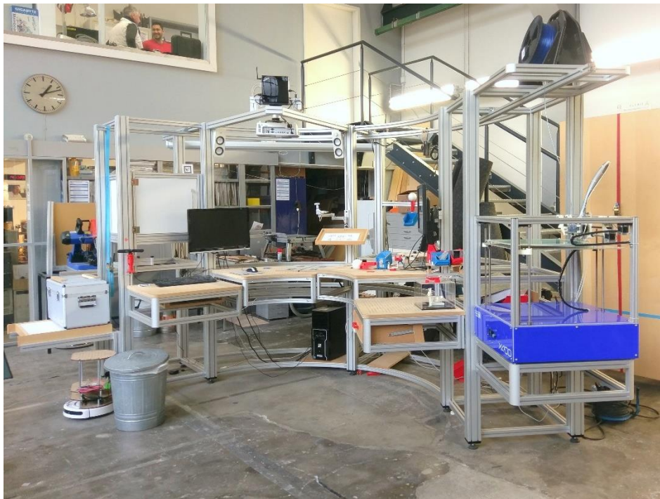
Figure 2-5: Prototype of USA 2 cloud manufacturing station
