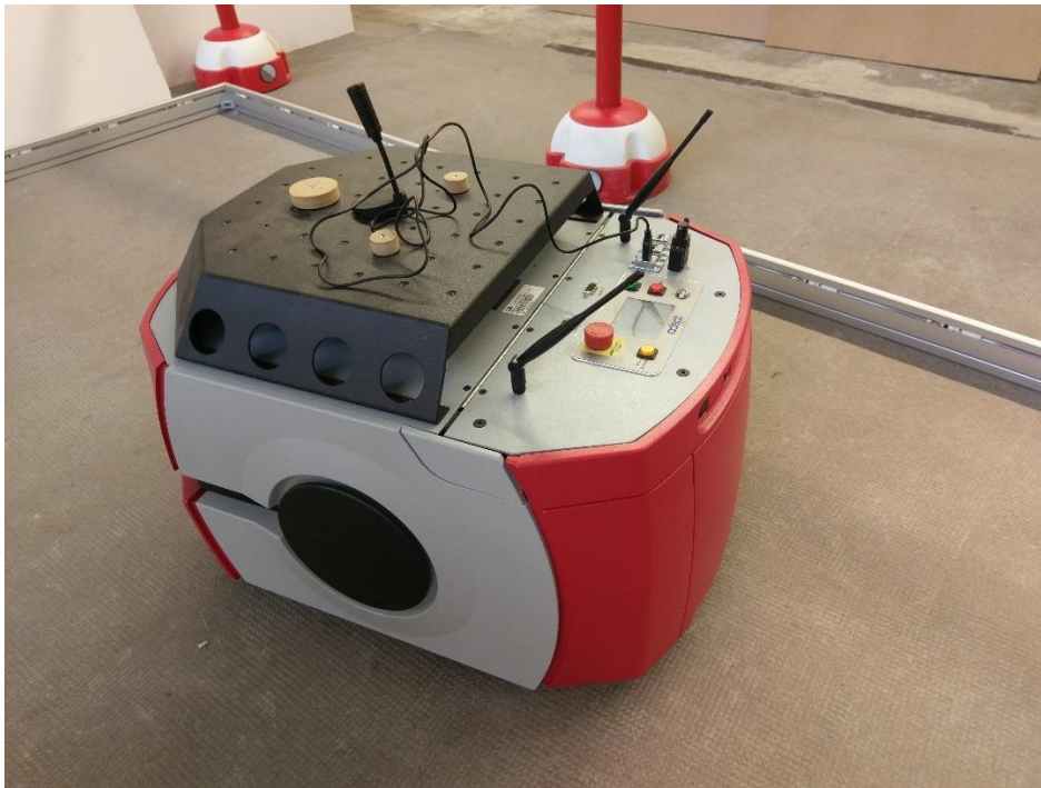
Figure 2-7: The assistive mobile robot in the infrared fall detection field
