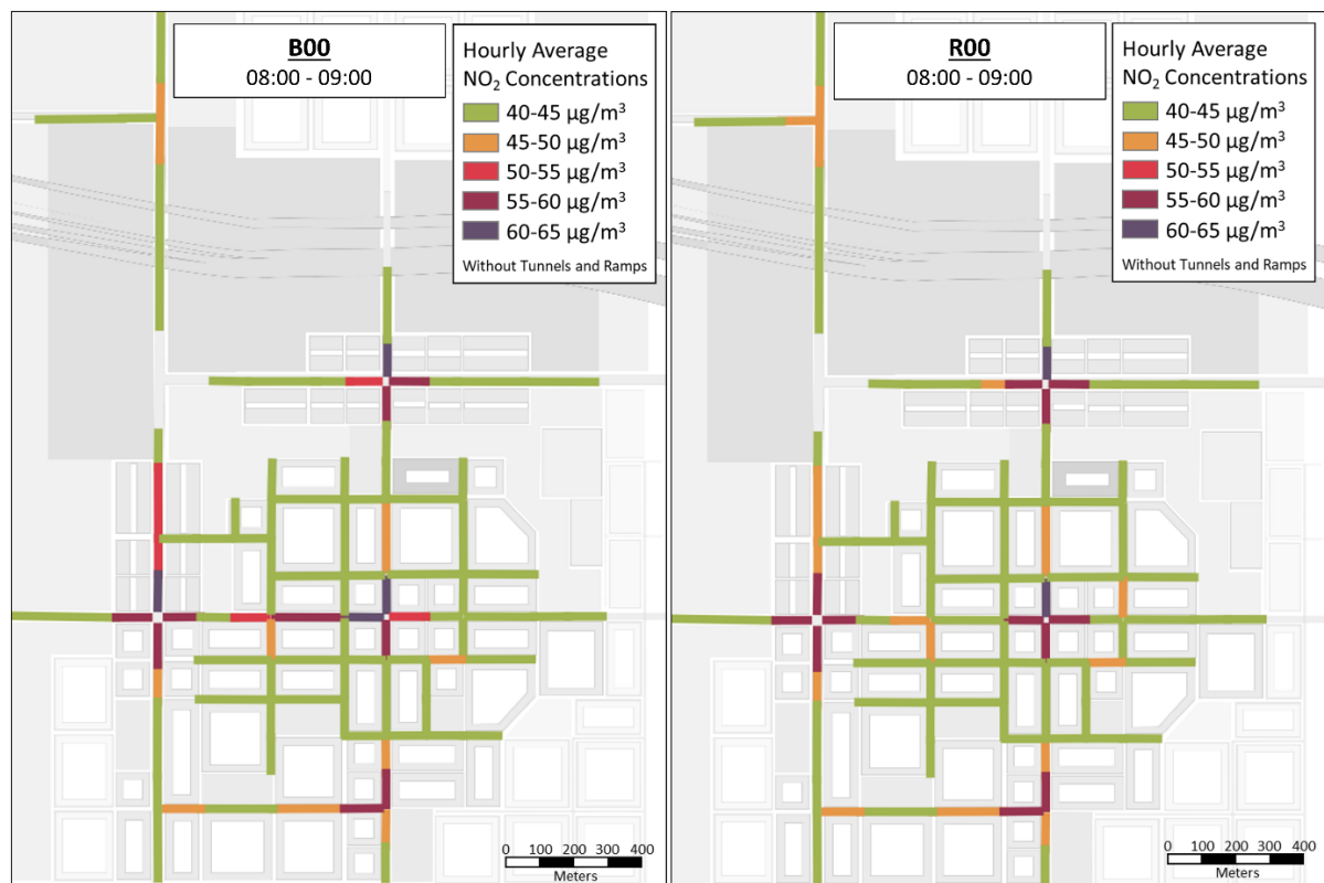
Figure 6.13 Comparison of \text{NO}_2 concentrations in base scenario (B00) and initial routing scenario (R00)
