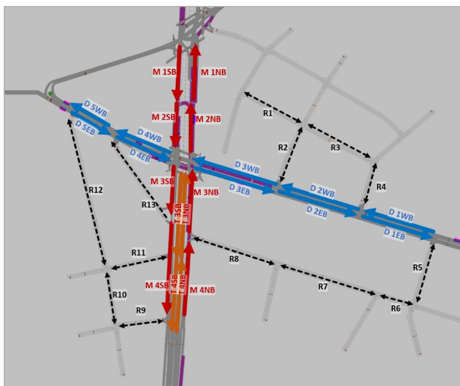
Figure 4.12 Microscopic traffic flow simulation network
