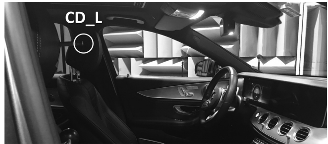
FIG. 4. The vehicle passenger cabin view in the anechoic chamber. The airborne measurement setup with the omnidirectional microphone is shown. The measurement position is head high on the left side of the co-driver seat (CD_L), and the microphone is mounted to the headrest.
