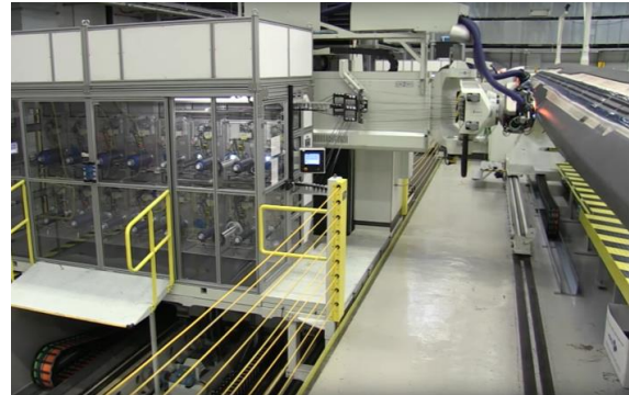
Figure 2.4: TS-AFP lay-up of a) Airbus A350 door surround structure at Premium Aerotec with a Coriolis Composites C1 [30], b) Airbus A350 wing skin with a MTorres TORRESFIBERLAYUP gantry machine [27, 31], c) Boeing 787 fuselage section at Spirit AeroSystems with a Electroimpact machine [32], d) Airbus A350 rear spar at GKN with a MTorres TORRESFIBERLAYUP column machine [33].
