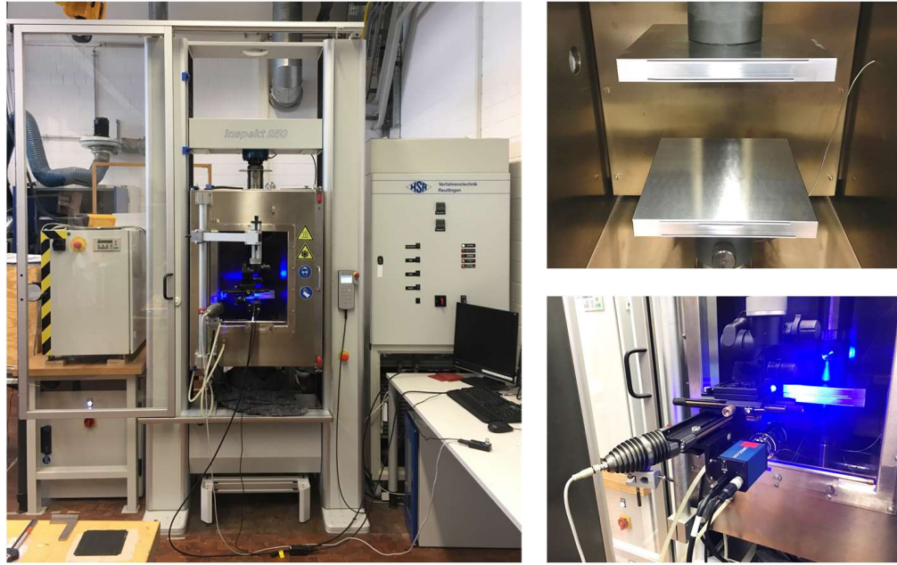
Figure 4.11: Experiment setup of the compaction experiments on the 250 kN universal testing machine (UTM) (left) with compaction plates (top right) and video extensometer (bottom right).
