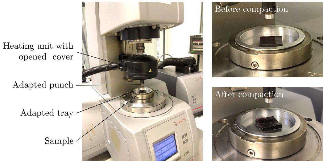
Figure 4.1: Experiment set-up of the rheometer compaction experiments with adapted punch cylinder, adapted tray and uncured prepreg standard samples before (top right) and after (bottom right) compaction.
