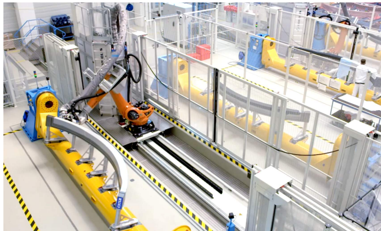
Figure 2.2: TS-AFP manufacturing of Airbus A350 door surround frames at Premium Aerotec frame center in Augsburg. [23]
