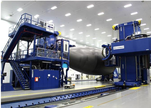
Figure 2.4: TS-AFP lay-up of a) Airbus A350 door surround structure at Premium Aerotec with a Coriolis Composites C1 [30], b) Airbus A350 wing skin with a MTorres TORRESFIBERLAYUP gantry machine [27, 31], c) Boeing 787 fuselage section at Spirit AeroSystems with a Electroimpact machine [32], d) Airbus A350 rear spar at GKN with a MTorres TORRESFIBERLAYUP column machine [33].
